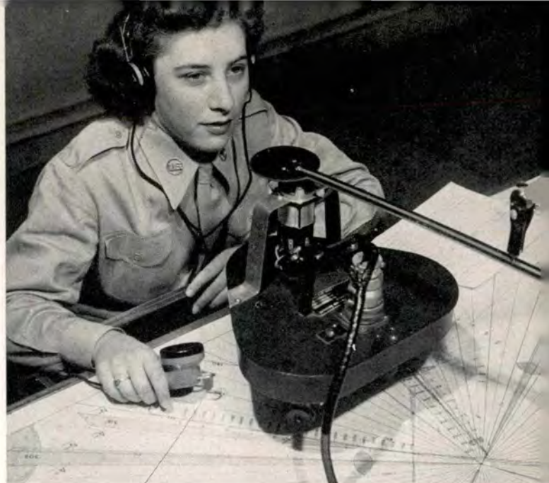
Link radio compass is automatically corrected by telemotor attachment to crab of the plotter. Operator is Pfc Mary Stewart.
